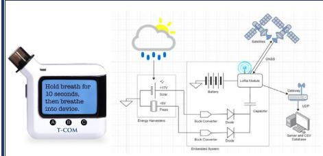
Range Wide-Area Network (LoRaWAN) or Narrowband Internet of Things (NB-IoT). The second objective is to allow this communication hardware to operate without human/manual intervention
