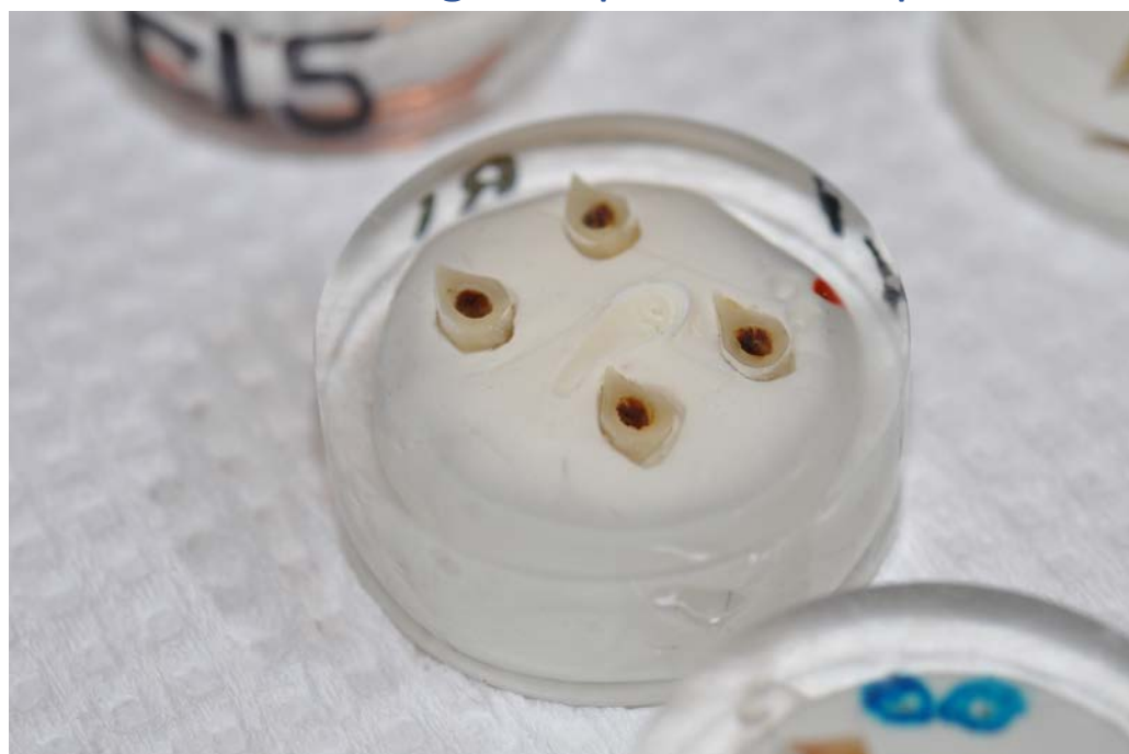
Figure 1- After embedding and sawing of the femoral head.
