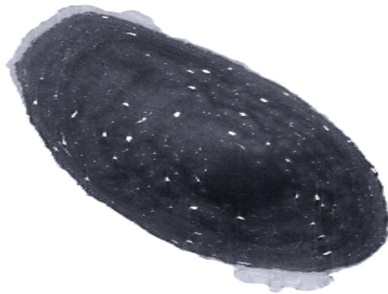
**Figure 1:** First image acquired of the nano-CT bone scans. The dark colors indicate bone and the white colors between the dark colors indicates pores.
