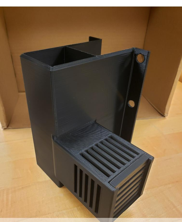
3D printed version of new particle imaging module.
