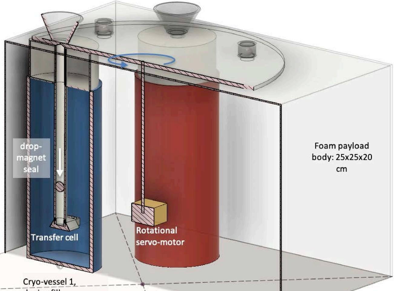
dry ice fill Cross-sectional schematic showing the ICE-Ball cryo-collection funnels and vessels that are filled with dry ice; they can seal cirrus particles in pristine condition for approx. 6 hours.
