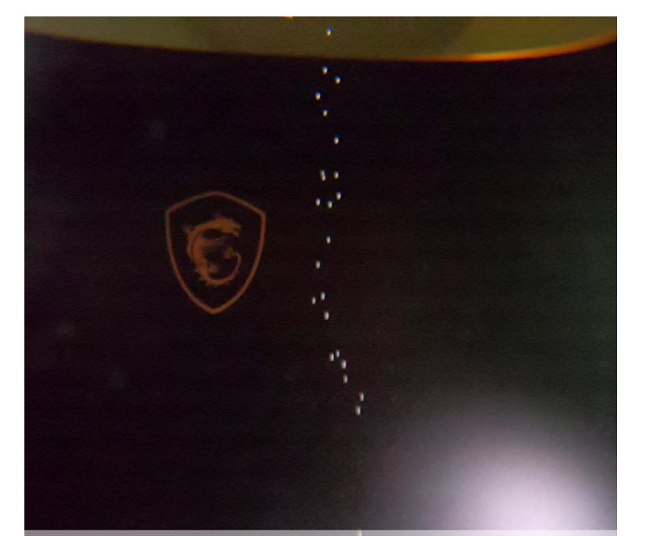
Successful imaging test of 500 micron glass beads using LumeCube illumication and new HD GoPro Hero8 action camera.
