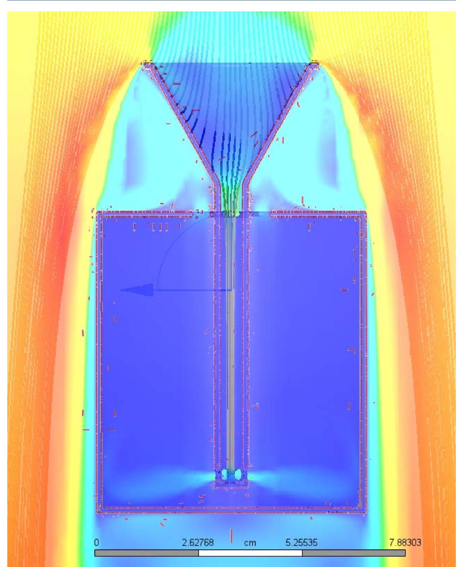
Computational Fluid Dynamics Simulation (CFD) of 5 m/s airflow past ice particle collection module. The model projects that including holes at strategic locations in the capture tube will allow efficient collection of smaller ice particles (minimum w/ no holes 50 microns vs. approx. 25 microns w/ holes).
