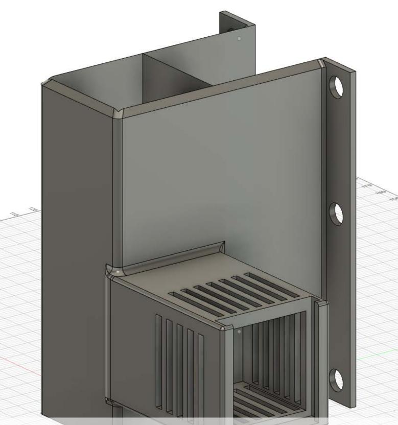
3D design for new particle imaging system. Designed in Autodesk Fusion, allowing for direct 3D printing.
